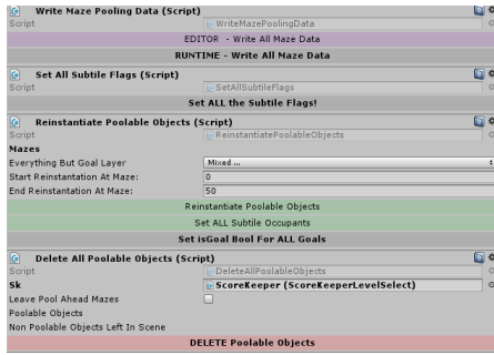
Figure 8: Pool Party Tools - when a designer is happy... with their maze changes, they use the "Write" tool to save all relevant data to JSON, 6 then use the "Delete" script to clear the Scene of all poolable objects. Nearly emptying the Scene enables faster load times 7 . When additional changes are needed, running the "Reinstantiate" script re-populates the Scene from JSON, ready to edit!
